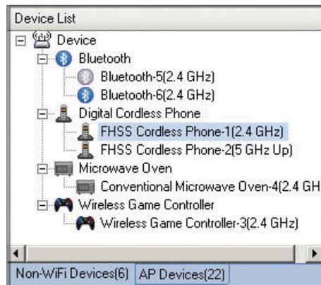
Figure 4: Detect and classify interfering sources
