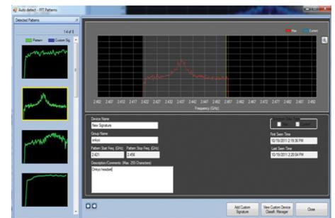
Figure 3: Automated detection of any RF interference source
